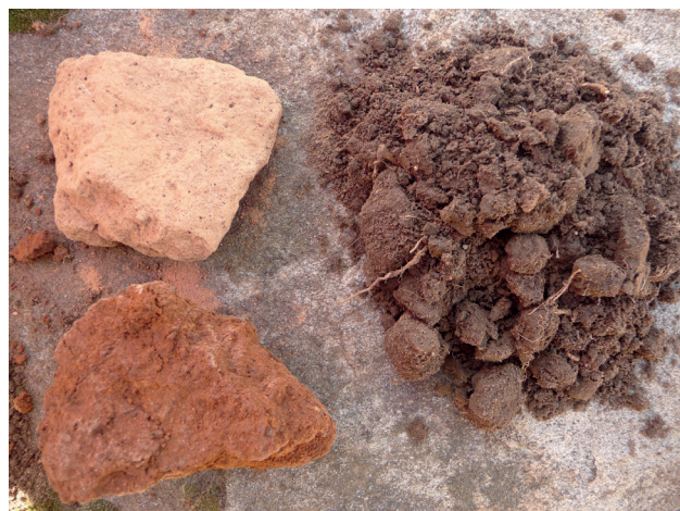
Figure 2: Compacted (left) and friable soil (right). (Source: A. Fox 2010)
