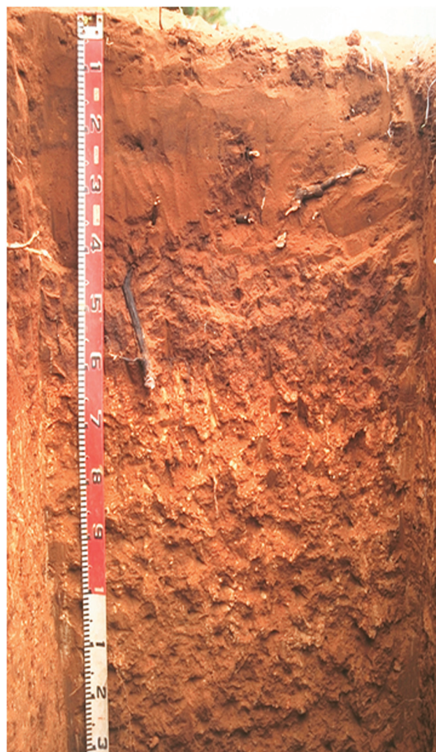
Figure 2 (left): Sandy loam over red clay. A soil profile on the Northern Adelaide Plains. (Source: D. Maschmedt 2009)
